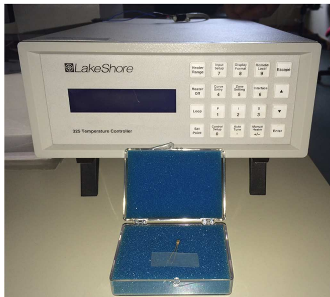
Fig. 4. LakeShore temperature measurement system. On the blue box, the calibrated diode.
